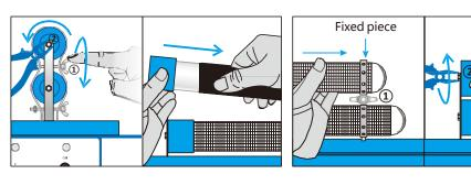
1.Twist the screw ① a few times counterclockwise, then fix the screw ② with pliers, twist a few times counterclockwise to remove the ion tube, and then remove the metal outer net.
