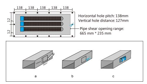
1.If the space is not enough, the equipment can't be installed in the pipe, please see the other install method below
