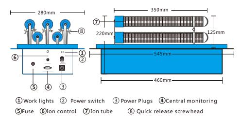
Note: Unplug the power before operation! This method is suitable for quickly replacing the ion tube without replacing the metal mesh.
