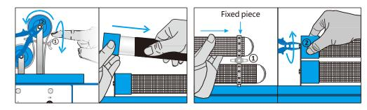
1. Twist the screw (1) a few times counterclockwise, 2.Put the new ion tube into the fixing clip, then fix the screw (2) with pliers, twist a few times tighten the screw (1), and then clamp the counterclockwise to remove the ion tube, and screw (2), and turn it clockwise a few then remove the metal outer net. times to replace the ion tube.
