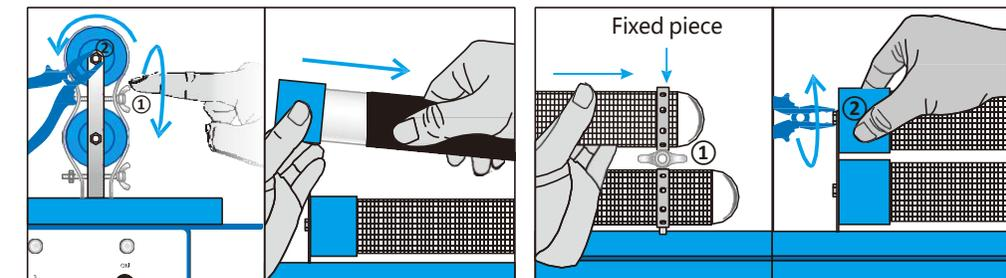
1. Twist the screw ① a few times counterclockwise, then fix the screw ② with pliers, twist a few times counterclockwise to remove the ion tube, and then remove the metal outer net.
