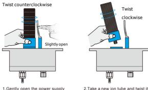
1.Gently open the power supply presser, pinch the ion tube, twist it counterclockwise several times, and then take it out.
